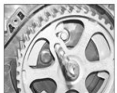
3.9 Insert a 5mm drill bit through the hole in the crankshaft sprocket into the cylinder head.
