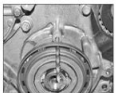
3.8 Insert a 5mm drill bit through the crankcase into the crankshaft sprocket hole in the oil pump housing (blue lining ball cover removed for clarity).
